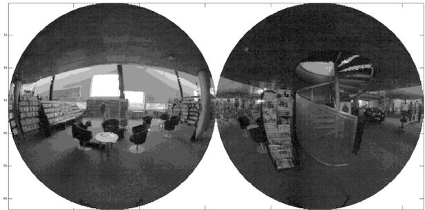
Figure 3. Two luminance maps (calibrated photographs) captured with a 180° equisolid-angle fisheye lens, from the same point, facing opposite directions. (logarithmic scale)
